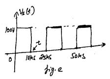
The input waveform for the above circuit (fig.e) is given in (fig.f). The circuit contains a non-ideal diode with following parameters.
